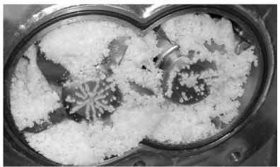
Figure 3: Rubber Crumble Formation in Finisher
