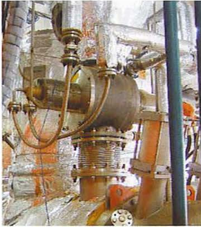
Fig. 5 Volumetric pulp feeder into vacuum
