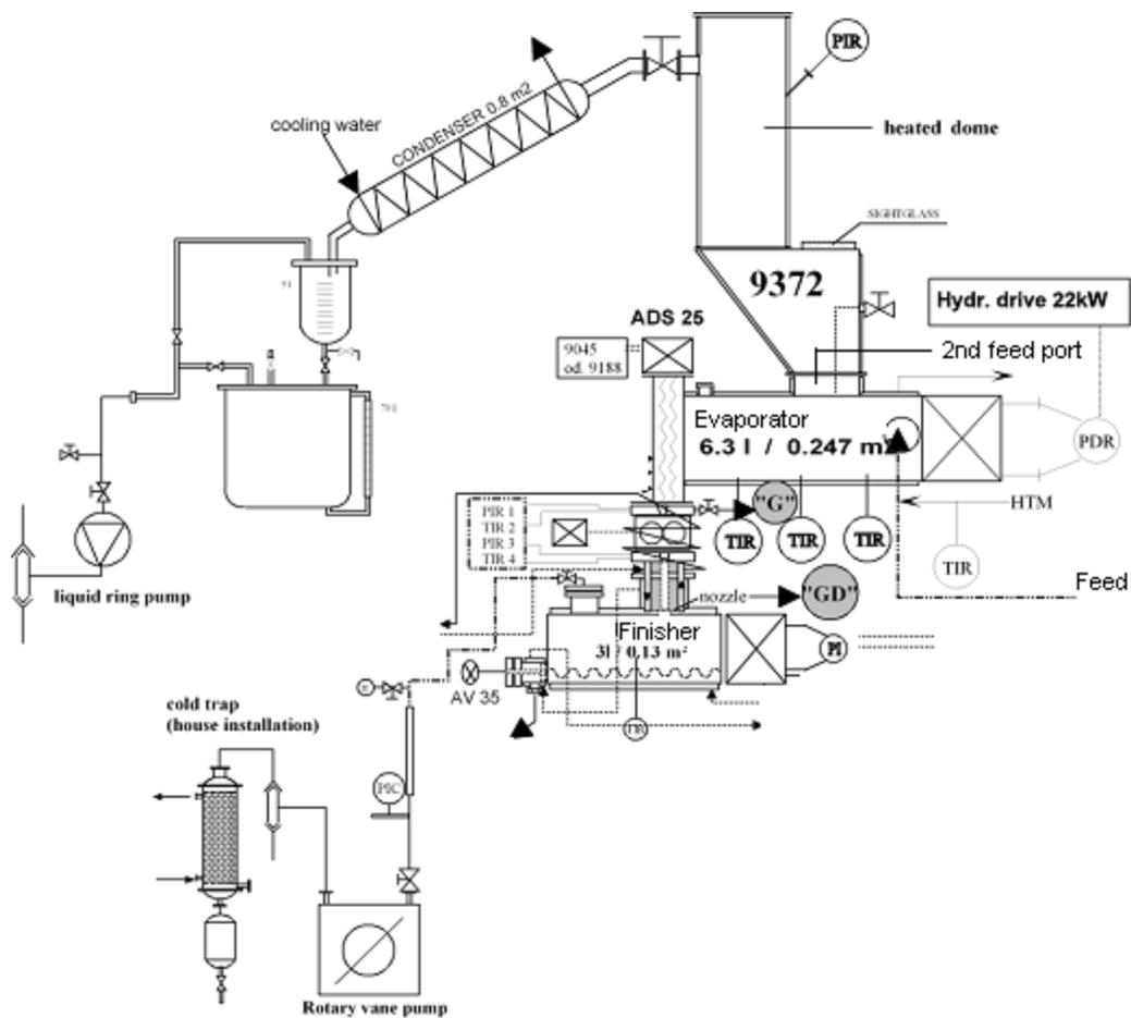
Figure 4: Test set up for evaporation trial
