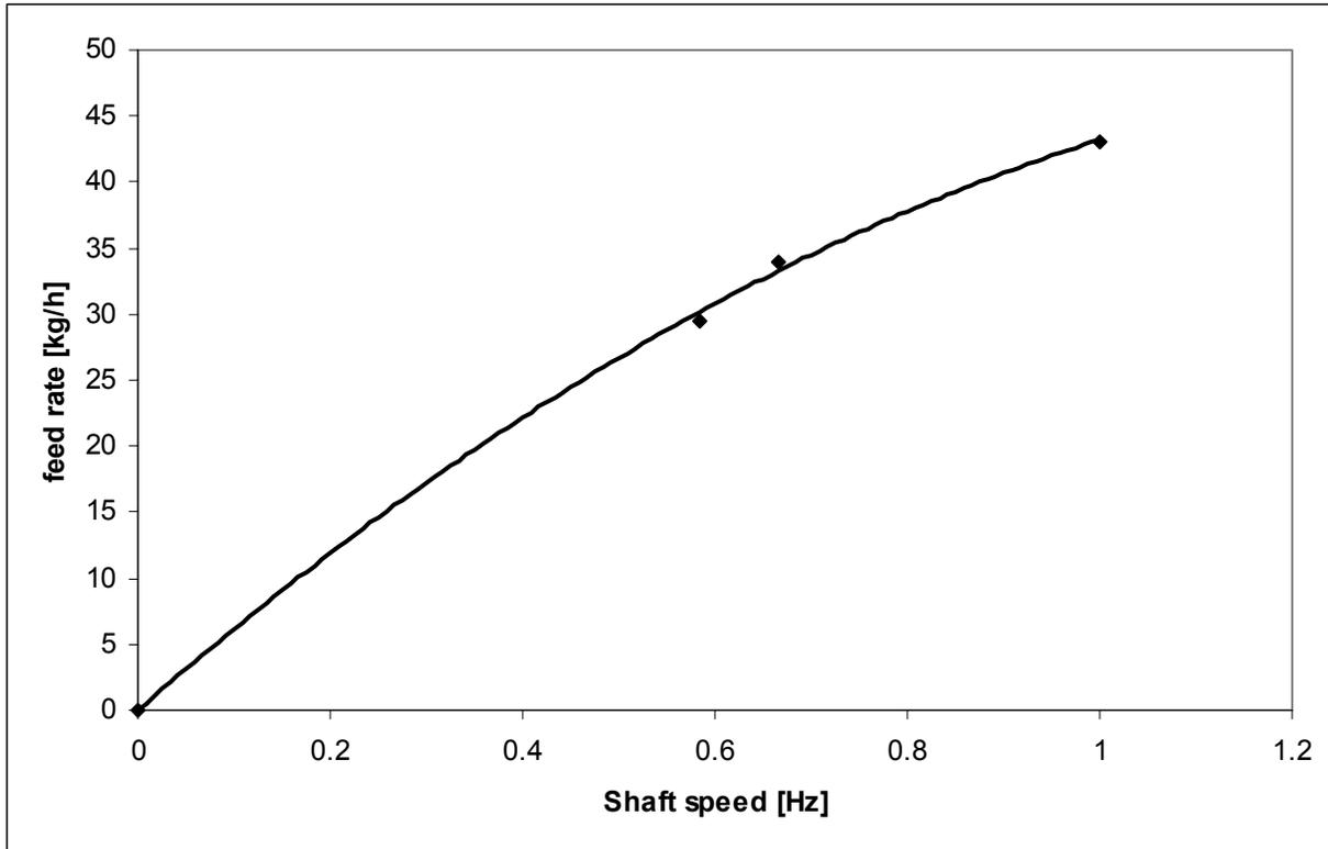
Figure 7: Cement feed rate versus kneader main shaft speed
