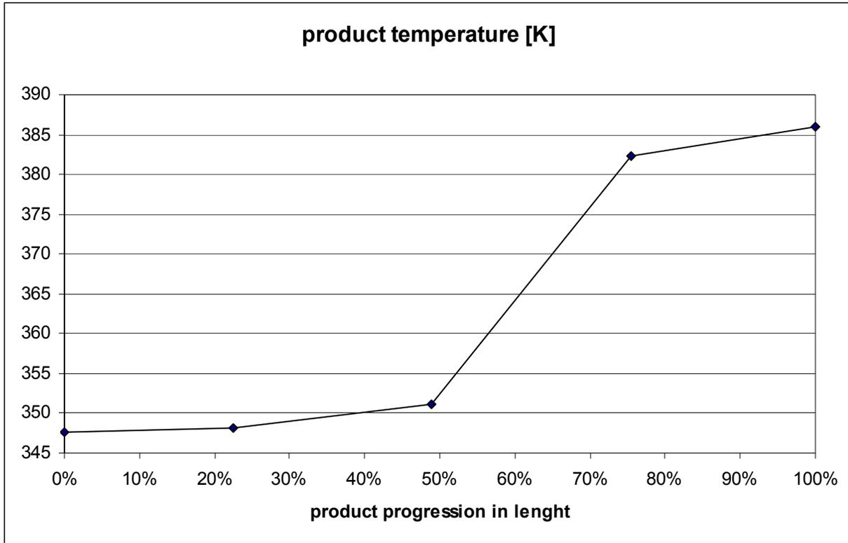
Figure 5: Temperature profile in kneader evaporator
