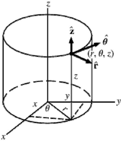
Figure 1: Cylindrical coordinates,  $z$  would be the main transport direction, which is horizontal in kneaders and extruders. The radial direction is described by  $r$  and the tangential direction by  $\theta$
