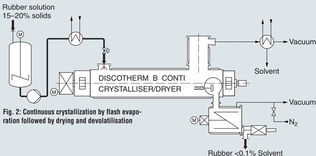
Fig. 2: Continuous crystallization by flash evaporation followed by drying and devolatilisation
