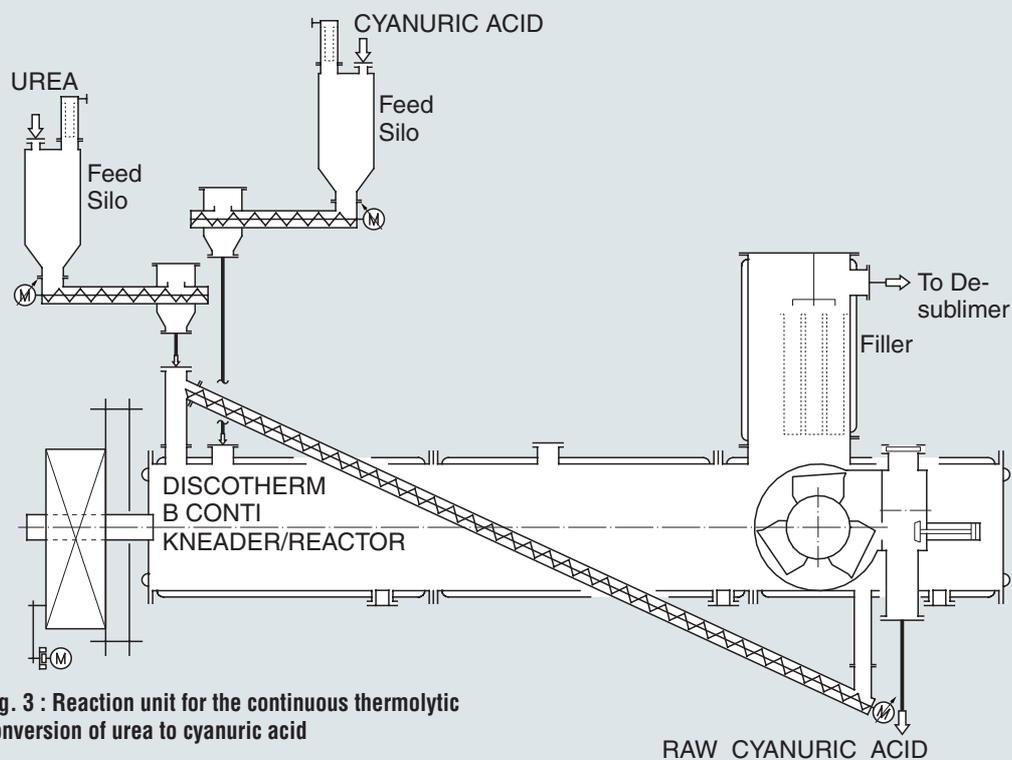
Fig. 3 : Reaction unit for the continuous thermolytic conversion of urea to cyanuric acid
