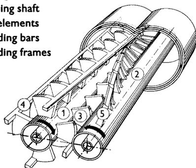
Figure 1. All-Phases Kneader-Dryer
