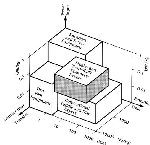
**Figure 3. Positioning of Kneaders-Dryers**
