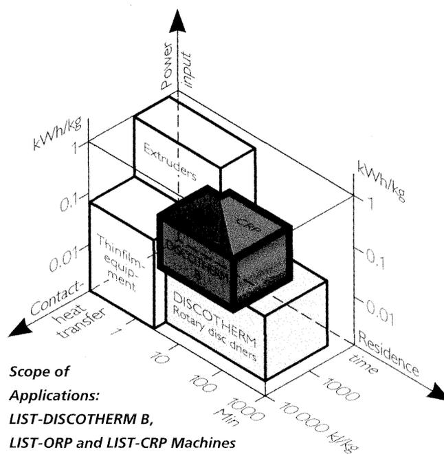
**Mixing & Kneading with Visous, Pasty and Granular Materials**
