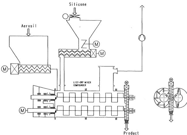
**Mixing/Compounding of Silicone with Aerosil**
