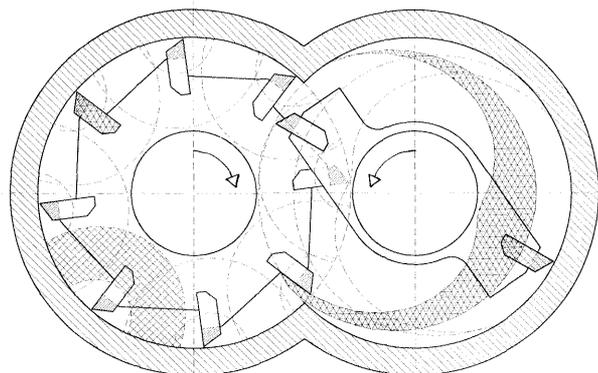
Fig. 1 Flow pattern and self-cleaning effect in ORP
