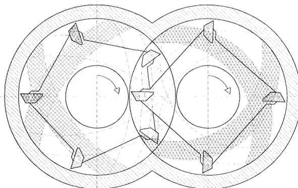
Fig. 2 Flow pattern and self-cleaning effect in CRP
