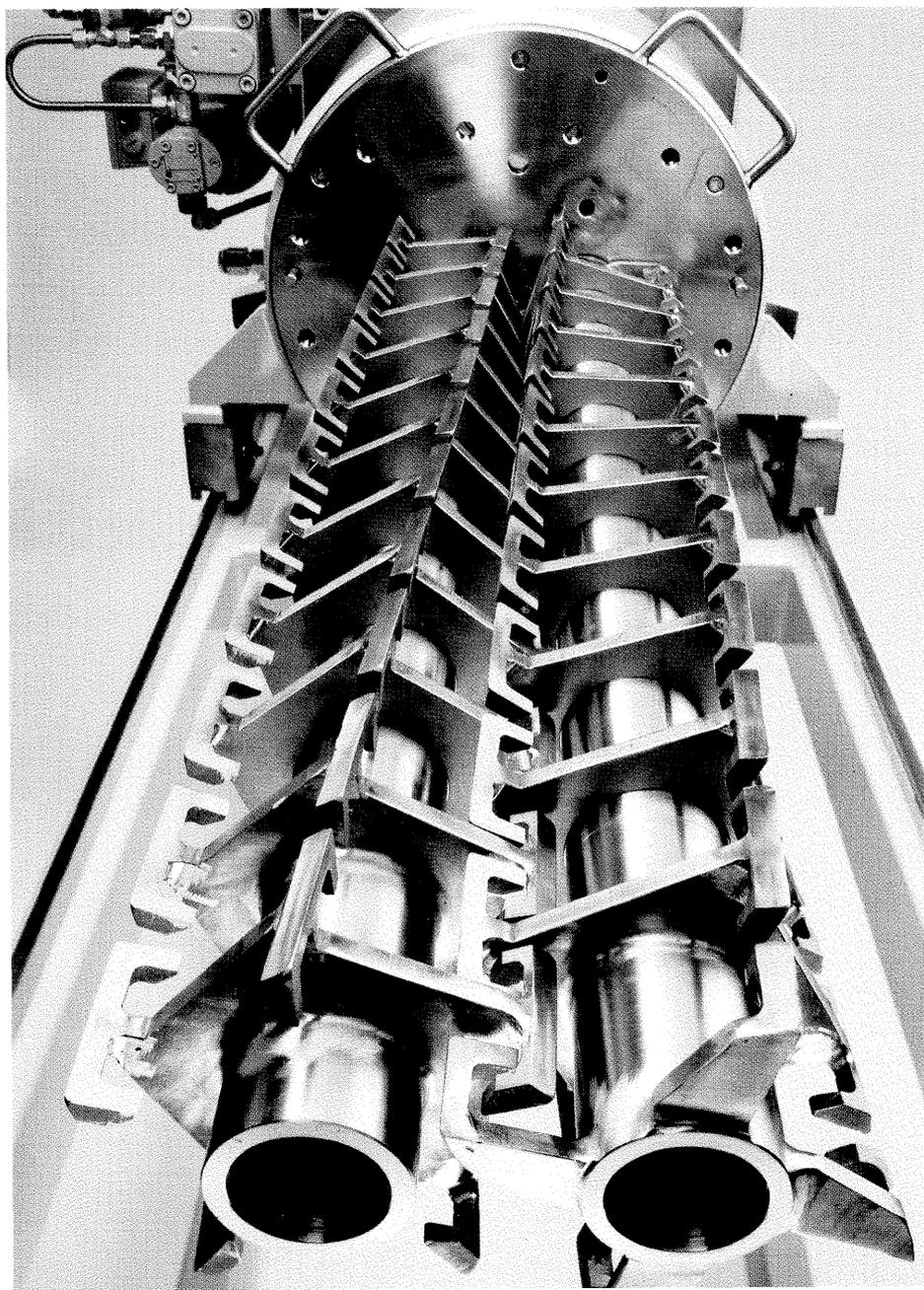
Fig. 3 Agitator shafts of CRP
